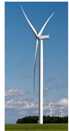
N117/2400 Gamma (2,4 MW, Fa. Nordex)
